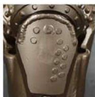
Shirrtail protection with tungsten carbide inserts
