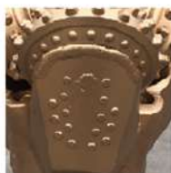
Shirrtail protection with tungsten carbide inserts
