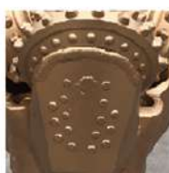
Shirttail protection with tungsten carbide inserts
