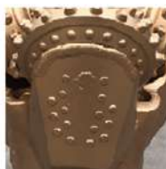
Shirrtail protection with tungsten carbide inserts
