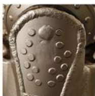
Shirrtail protection with tungsten carbide inserts
